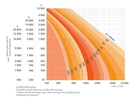
**Note:** Information based on normal load conditions, using age resistant average quality grease, +70°C (+158°F) bearing temperature.
